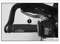
Clutch lever **1** is fitted on the handlebar on the left. The clutch is activated hydraulically and adjusts itself automatically.
