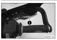
The hand break lever ① is fitted on the right side of the handlebar.
