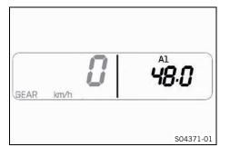
Press the + or - button repeatedly until A1 is shown on the combination instrument.
