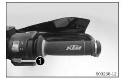
Start button **()** is fitted on the right side of the handlebar.
