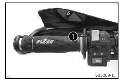
The light switch ① is fitted on the left side of the handlebar. **Possible states**
