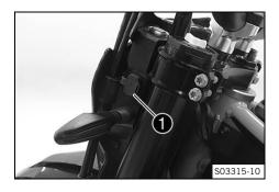
A USB socket ① for supplying power to external devices is located on the left side of the headlight mask. The USB socket is activated when the ignition is switched on.
