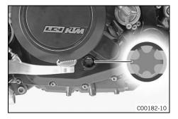
Check the engine oil level.
