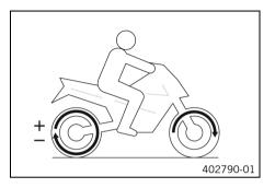
The slip adjustment is an optional motorcycle traction control function.
