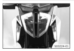
The cornering light is located on the left and the right in the fuel tank spoiler.
