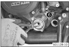
Pull oil filter 6 out of the oil filter housing.
