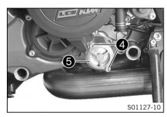
Remove screws **4**. Take off oil filter cover **5** with the Oring.
