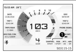
The **Damping** mode setting is shown in the **1** area of the display. The damping can be configured in the **Motorcycle** menu under **Damping**.
