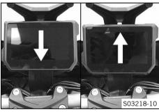
To move the combination instrument to the desired position, press combination instrument upward or downward.
