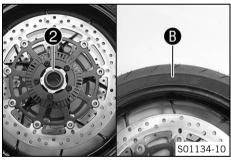
Insert wide spacer 2 on the left in the direction of travel.
