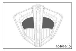
The low beam is integrated in the main headlight. The low beam is activated when the ignition is switched on. To save power in the 12-V battery, the low beam is deactivated again after 5 seconds if the engine is not started. If the ignition is accidentally switched off during the journey, the low beam remains on.
