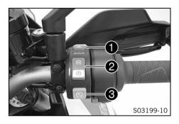
The right combination switch is fitted on the right side of the handlebar.
