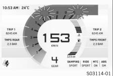
The shift warning light is integrated in the tachometer display. In the **Settings** menu under **Shift Light**, the engine speed for the shift warning light can be set. The shift warning light is always active during the running-in phase (up to 1,000 km / 621 mi). The shift warning light can only be deactivated, and the values for **Shines** and **Flashes** can only be adjusted after this. The shift warning light lights up red at **Shines** and flashes red at **Flashes**.
