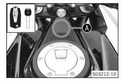
On this vehicle, the ignition/steering lock is replaced by a remote key with transponder (RACE-ON key () p. 43)).
