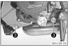
Mount and tighten oil drain plugs 3 with magnets, O-rings, and oil screens.
