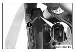
A USB socket **1** for supplying power to external devices is located in the left storage compartment.
