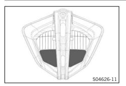
The high beam is integrated in the main headlight.
