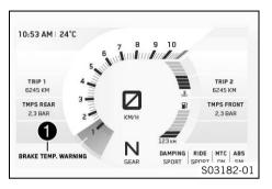
When the rear brake is used frequently and for excessively long periods, for example on long downhill stretches, the temperature of the brake system may increase.
