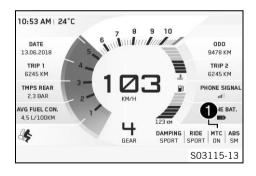
The **1** area of the display indicates whether **MTC** the system is switched on or off.
