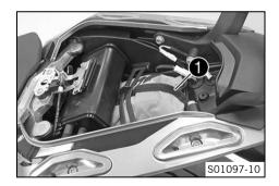
The storage compartment under the passenger seat contains tool set 1.
