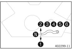
The gear positions can be seen in the figure. The idle position is between first and second gears.
