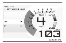
The **Anti Wheelie Mode** is an optional vehicle electronics function. Anti wheelie mode is intended to prevent the front wheel rising when accelerating.
