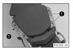
Case holders are located on each side of the passenger seat. A case system (optional) can be attached on the case holders. The case holders may not be loaded with more than the specified weight.
