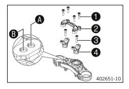
Remove screws **1**. Take off handlebar clamp **2**. Take off handlebar and place it to the rear.
