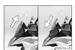
To move the windshield to the desired position, push the windshield upward or downward.
