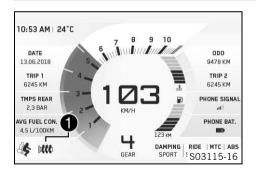
When the heated grip is activated, the **Heated Grips** symbol appears in the **1** area of the display.
