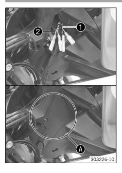
The front power supplies ACC1 1 and ACC2 2 are located on the right side of the instrument support behind a cover 1.
