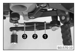
Loosen nut 1, holding threaded rod 2.
