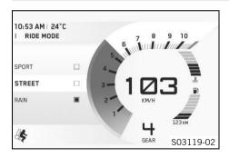
When the menu is closed, **Quick Selector 2** is opened by pressing the **DOWN** button.
