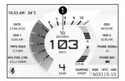
The operating state and active cruise control are shown in the **1** area of the display.
