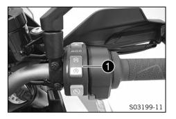
The start button/emergency OFF switch is fitted on the right side of the combination switch.
