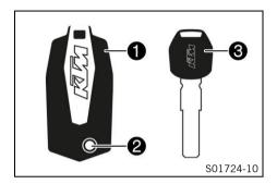
In this vehicle, the  $\underline{RACE-ON\ key}$   $\bigcirc$  performs all the functions of the conventional ignition key.
