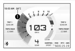
The ambient air temperature is displayed in the **1** area. The units of the ambient temperature can be configured in the **Settings** menu under **Units**.
