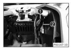
The rear power supplies ACC1 1 and ACC2 2 are located on the right next to the passenger seat lock.
