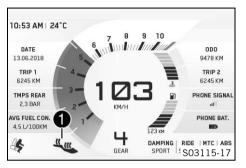
When the seat heating is activated, the **Heated Seat** symbol appears in the **1** area of the display.
