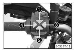
The menu switch is fitted in the middle on the left side of the combination switch.
