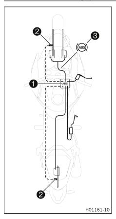
The ABS module ①, which consists of a hydraulic unit, ABS control unit, and return pump, is installed on the right side of the vehicle below the fuel tank. One wheel speed sensor ② is located in each case on the front and the rear wheel.
