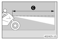
Position the vehicle perpendicular to the wall at a distance **(6)** from the wall and switch on the low beam
