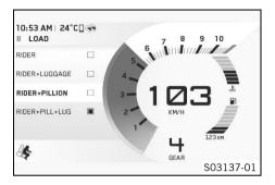
When the menu is closed, **Quick Selector 1** is opened by pressing the **UP** button.
