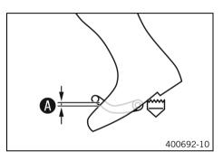
Sit on the vehicle in the riding position and determine distance between the upper edge of your boot and the shift lever.
