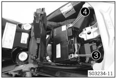
Position positive cable 3, mount and tighten screw.
