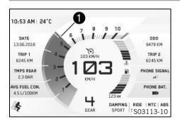
The engine speed is shown in area **1** of the display. The engine speed is measured in revolutions per minute.
