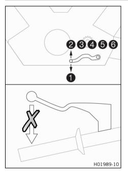
If the <u>quickshifter +</u> (optional) is activated, you can shift up and down without actuating the clutch.
