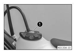
Press release button 1, turn the fuel tank filler cap counterclockwise, and lift it off.
