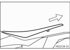
Raise the rear of the seat, pull the seat back, and lift it off.
