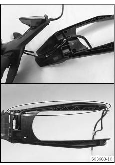
Position the tail light together with the license plate holder on the license plate bracket.
