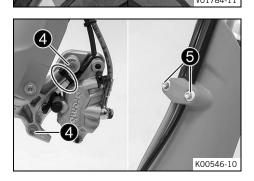
Position the brake caliper, and mount and tighten screws 4.
