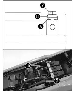
Connect the positive cable to the 12-V battery.
