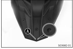
Drill a hole at marking A on the license plate holder to the size of the marking.
