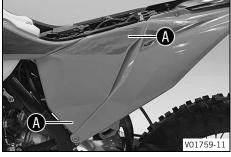
Pull off the air filter box cover in area (A) laterally and take it off at the front.
