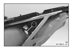
Disconnect tail light plug-in connector on the wiring harness
