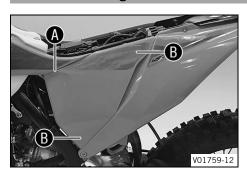
The air filter box cover is secured.
