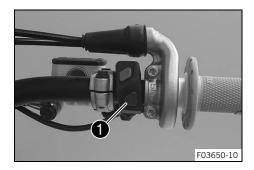
Start button **1** is fitted on the right side of the handlebar.
