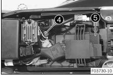
Pull up the battery holding bracket 6 and remove the 12-V battery to the rear.
