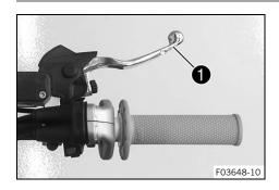
Hand brake lever **1** is fitted on the right side of the handlebar. The front brake is engaged using the hand brake lever.
