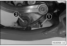
Mount and tighten screw plug 3 with the O-ring.
