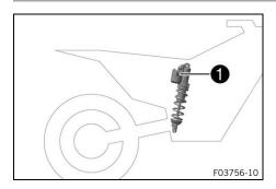
The shock absorber article number **1** is stamped on the top of the shock absorber.
