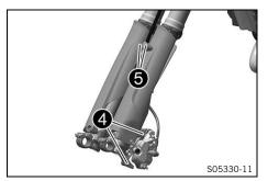
Position the brake caliper. Mount and tighten screws 4.
