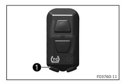
Press the TC button 1 to switch traction control on or off.
