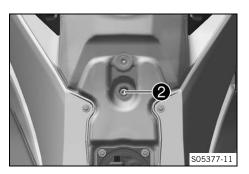
Mount and tighten screw with the rubber bushing.
