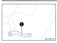
Foot brake lever **1** is located in front of the right footrest. The foot brake lever is used to activate the rear brake.
