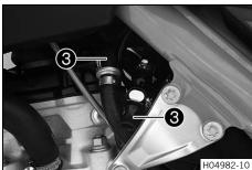
Disconnect the quick release coupling.
