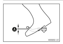
Sit on the vehicle in the riding position and determine distance between the upper edge of your boot and the shift lever.
