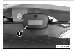
The combination instrument **1** is attached in front of the handlebar.
