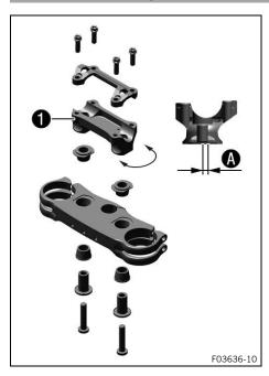
The holes on the handlebar support  $\mathbf{1}$  are placed at a distance of  $\mathbf{A}$  from the center.
