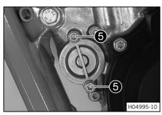
Remove screws 6. Take off the oil filter cover with the Oring.
