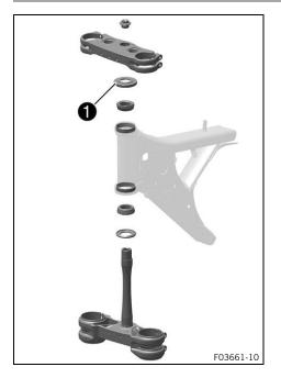
Clean the bearing and sealing elements, check for damage, and grease.
