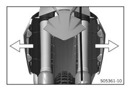
Pull both spoilers laterally off the radiator and lift off the fuel tank.
