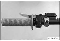
Position the controls on the left handlebar half.
