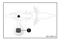
The diagnostics connector **1** is located under the seat below the EFI control unit.
