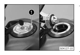
Lift cover 1 of the fuel tank filler cap and insert the ignition key into the lock.
