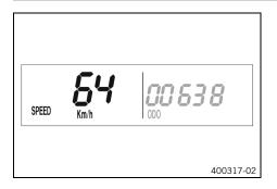
The current speed is displayed in the **SPEED** display mode. The current speed can be displayed in **Km/h** or **Mph**.
