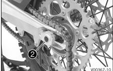
✓ The brake linings are correctly positioned.
