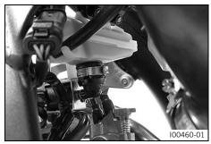
Insert the oil screen and mount the angle piece with a new hose clamp.
