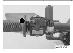
Horn button **1** is fitted on the left side of the handlebar.
