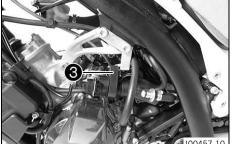
Remove fuel vapor valve 3 from the bracket and hang it to the side.
