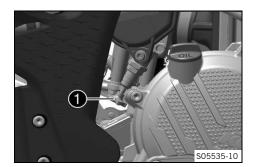
The cold start button **1** is fitted to the bottom of the throttle valve body.
