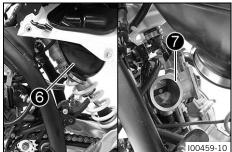
Lift the subframe slightly and secure it.
