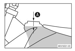
Fill the fuel tank with fuel up to a maximum of level A.
