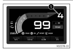
The current gear is shown in area **1** of the display.
