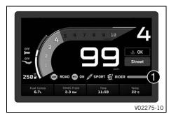
The payload setting is shown in area **1** of the display. The payload can be configured in the **Load** menu. Only configure the payload in an unloaded state.
