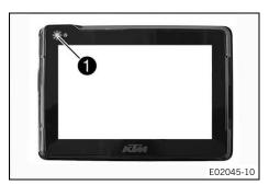
The immobilizer indicator lamp can indicate malfunctions by flashing. These are indicated up to five seconds after the unlock button is actuated.
