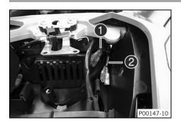
The rear power supplies ACC1 1 and ACC2 2 are located on the right next to the passenger seat lock.
