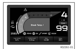
When the rear brake is used frequently and for excessively long periods, for example on long downhill stretches, the temperature of the brake system may increase.
