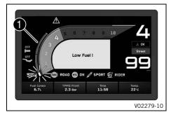
The fuel tank capacity is shown in area **1** of the display. The fuel level indicator consists of bars. The more bars are lit, the more fuel is in the fuel tank.
