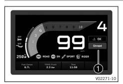
The **Ride Mode** setting is shown in area **1** of the display. The riding mode can be configured in the menu **Ride Mode**.
