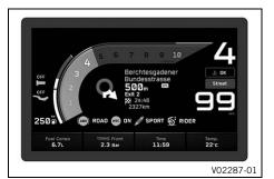
The **Navigation** indicator appears when the navigation function is activated
