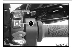
The <u>Unlock button</u> **1** is fitted on the right side of the combination switch.
