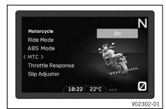
The motorcycle traction control ( $\underline{\text{MTC}}$ ) lowers the engine torque in case of loss of traction in the rear wheel.
