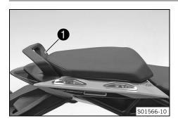
The passenger can hold onto the grab handle **1** during the trip.
