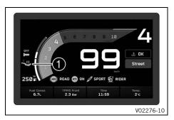
The status of the seat heating is shown in area **1** of the display. The seat heating can be configured in the **Heating** menu.
