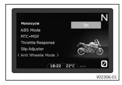
The **Anti Wheelie Mode** is an optional vehicle electronics function. Anti wheelie mode is intended to prevent the front wheel rising when accelerating.
