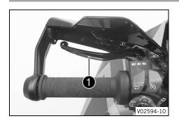
Clutch lever **1** is fitted on the handlebar on the left. The clutch is activated hydraulically and adjusts itself automatically.
