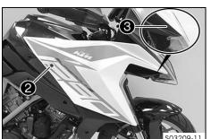
Mount and tighten screws 2 and 3.
