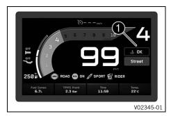
The coolant temperature is shown in area 1 of the display.
