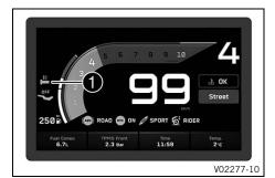
The status of the grip heater is shown in area **1** of the display. The grip heater can be configured in the **Heating** menu.
