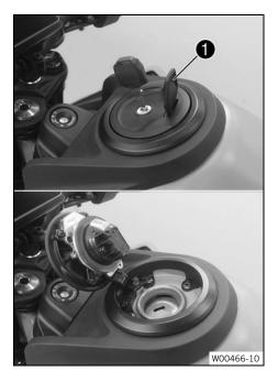
Lift cover of the fuel tank filler cap and insert the ignition key into the lock.
