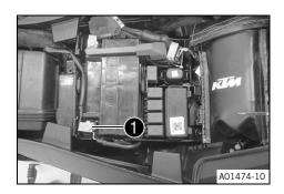
Disconnect negative cables of the 12-V battery.
