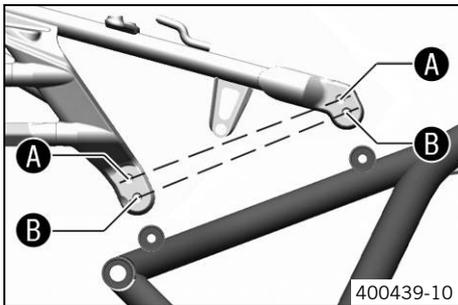
The subframe can be mounted in two different positions. This enables the seat to be positioned at an ergonomic height.
