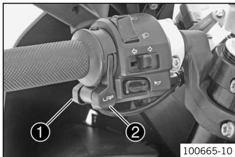
The **MODE** button ① is fitted on the handlebar, front left.
