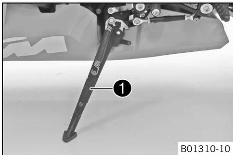
The side stand **1** is located on the left side of the vehicle. The side stand is used for parking the motorcycle.
