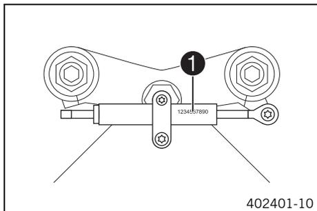
The steering damper part number ❶ is stamped on the top of the steering damper.
