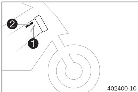
The vehicle identification number **1** is stamped on the frame behind the steering head on the right.
