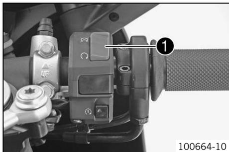
The emergency OFF switch ❶ is installed on the right side of the handlebar.
