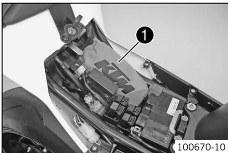
The tool set ❶ is in the storage compartment under the seat.
