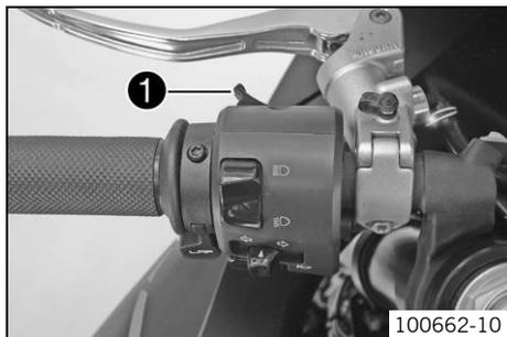
The headlight flasher switch ❶ is fitted on the left side of the handlebar.
