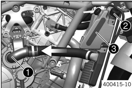
The water pump with a 3D water pump wheel ❶ in the engine ensures forced circulation of the coolant. The heat exchanger enables faster warming of the engine oil at the start of a journey and better heat dissipation for the engine oil during the journey.
