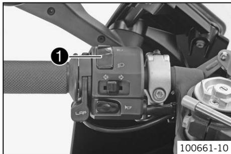
The light switch ❶ is fitted on the left side of the handlebar.
