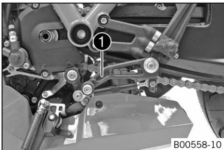
The shift lever **1** is mounted on the left of the engine.
