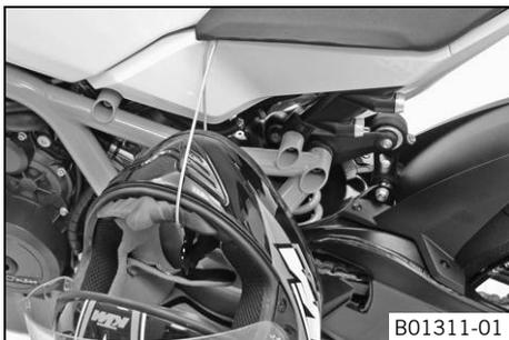
The steel cable in the tool set can be used to lock a helmet to the vehicle to prevent it from being stolen.
