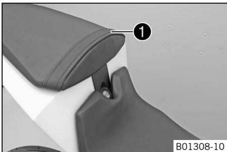
The supporting strap ❶ is provided for the passenger to hold on to.
