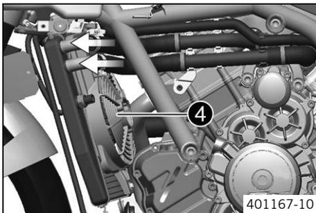
Cooling takes place by means of the air stream and a radiator fan ❹, which is controlled by a thermostat.
