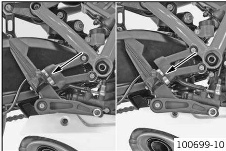
The adjustable footrest system enables an individual setting of the footrest height and an individual adjustment of the controls.
