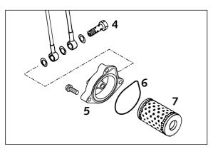
Check the O-ring for damage. O-rings need not be replaced unless damaged. Press the O-ring into the groove of the filter cover. Fit new oil filter with rubber gasket on the fitting in oil filter cover and mount cover with filter. Mount three screws and tighten with 5 Nm (4 ft.lb). Mount hollow screw with seal rings and tighten with 15 Nm (11 ft.lb). Start engine and check oil system for leakage.
