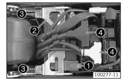
Slide the battery into the battery rack.
