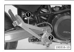
Position the footrest bracket ①. Mount and tighten screws ②.
