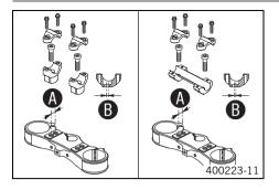
On the upper triple clamp, there are two holes a distance of **@** apart.
