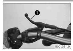
The choke lever **1** is fitted on the left side of the handlebar.
