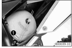
Put in both parts together, position them, and fix them with air filter holder ①.
