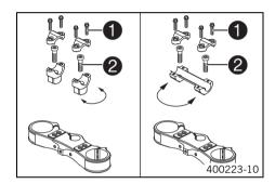
Remove the four screws ①. Remove the handlebar clamp. Remove the handlebar and lay it to one side.
