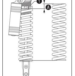
Depending on the static sag and/or the riding sag, it may be necessary to increase or decrease the spring preload.
