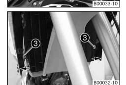
Pull both spoilers off of the sides of the radiator bracket 3 and lift off the fuel
