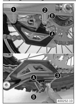
Remove screws • and •. Take off the chain guide.
