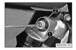
Turn adjusting screw • clockwise with a screwdriver to the last click.
