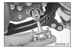
Mount the desired auxiliary spring and adjusting spring and slide them into the clutch cover together.
