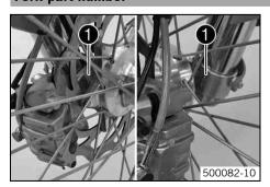
The fork part number  $oldsymbol{0}$  is stamped on the inner side of the fork stub.
