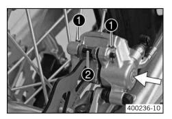
Press the brake caliper onto the brake disc by hand in order to push back the brake piston.
