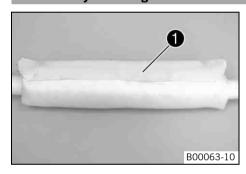
The main silencer is filled with glass fiber yarn  $\bullet$ .
