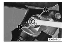
Turn adjusting screw ● all the way clockwise with a ring wrench.
