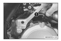
Remove screw cap • and fill up gear oil.
