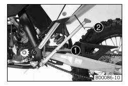
When you are riding, side stand • must be folded up and secured with rubber band •.
