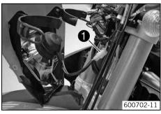
– Connect the electric plug connector lacktriangle.
