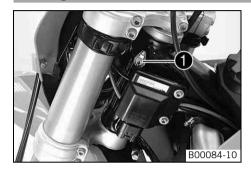
Steering lock • is fitted on the left side of the steering head. The steering lock is used to lock the steering. Steering, and therefore riding, is no longer possible.
