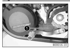
The engine number  $\ensuremath{\mathbf{0}}$  is stamped on the left side of the engine under the engine sprocket.
