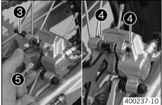
Insert the brake linings, insert bolt 3, and mount locking split pins 4.
