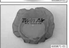
Mount the dust cover for the air filter.
