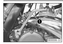
The kickstarter lacktriangle is fitted on the right side of the engine. The top part can be swiveled.
