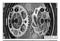
Clean and grease shaft seal rings • and bearing surface • of the spacers.
