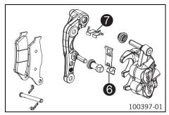
Check that leaf spring **⑤** in the brake caliper and sliding plate **⑦** in the brake caliper support are seated correctly.
