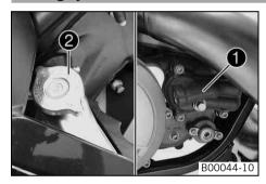
Water pump • in the engine circulates the coolant.
