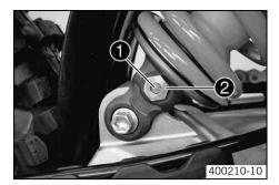
Turn adjusting screw 1 clockwise with a screwdriver to the last click.
