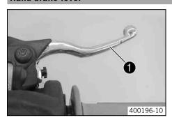
Hand brake lever **1** is located on the right side of the handlebar. The hand brake lever is used to activate the front brake.
