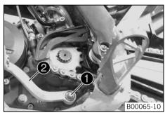
Remove screw 1 and remove shift lever 2.
