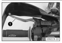
The clutch lever  $\bullet$  is fitted on the left side of the handlebar. The clutch is hydraulically operated and self-adjusting.
