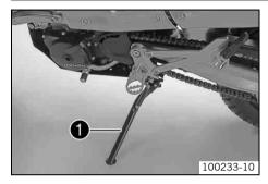
The side stand  ${\pmb 0}$  is coupled with the safety electric starter system - see the riding instructions.
