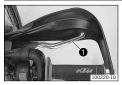
The hand break lever  $\bullet$  is fitted on the right side of the handlebar. The hand brake lever operates the front brake.
