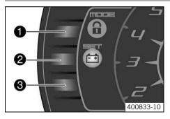
You can change the display mode with the **MODE** button **①**. Possible display modes are distance traveled (**ODO**), trip master 1 (**TRIP 1**) and trip master 2 (**TRIP 2**).
