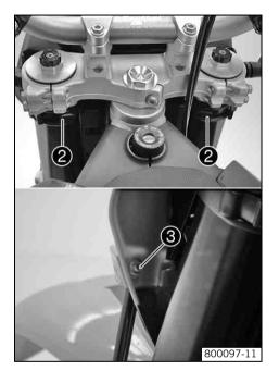
Position the headlight mask and fix it with rubber band ②.
