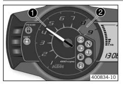
The tachometer **1** shows the engine speed in revolutions per minute. The red marking **2** shows the excess speed range of the engine.
