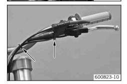
Position the controls on the left half of the handlebar.
