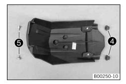
Insert the rubber sleeves 4 in the footrest bracket.
