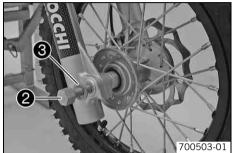
Hold the front wheel and pull out the wheel spindle ② with the washer ③. Take the front wheel out of the fork.
