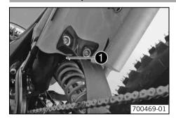
The shock absorber part number **1** is stamped on the top of the shock absorber above the adjusting ring towards the rear.
