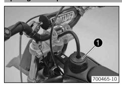
Turn the tank cap • counterclockwise and pull it up.
