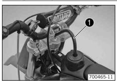
Put the tank cap on and turn it clockwise.
