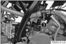
Pull the main silencer off of the manifold at the rubber sleeve 3.
