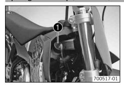
Turn the oil tank cap ① counterclockwise and pull it up.
