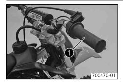
Throttle grip • is fitted on the right side of the handlebar.
