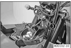
Disconnect the electrical plug-in connection 3 and remove the headlight mask with the headlight.
