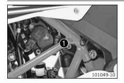
The seat can be released using strap **①**.
