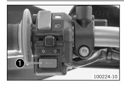
The horn button • is fitted on the left side of the handlebar.
