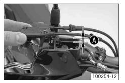
Adjust the brake fluid level to level **3**.
