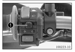
The turn signal switch • is fitted on the left side of the handlebar.
