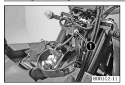
Connect the electrical plug-in connection •.
