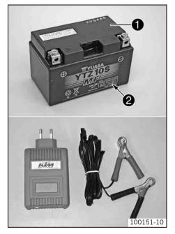
Connect the battery charger to the battery. Switch on the battery charger.
