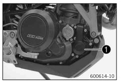
The water pump **1** in the engine forces the coolant to flow.
