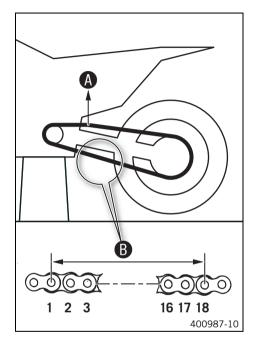
Pull on the upper section of the chain with the specified weight **a**.
