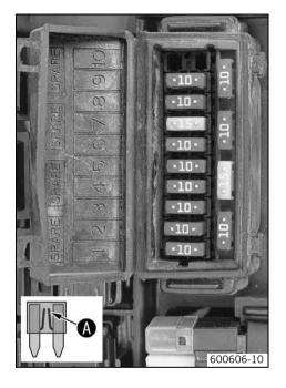
Remove the defective fuse.
