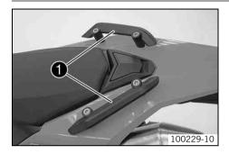
The handrails **①** are used for moving the motorcycle around. When you have a passenger, the passenger can hold on the handrails during the journey.
