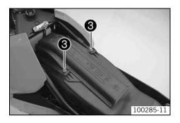
Mount and tighten screws 3.
