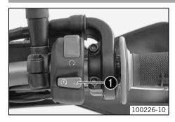
The electric starter button • is fitted on the right side of the handlebar.
