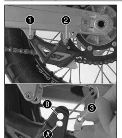
Remove screws • and •. Take off the chain guide.
