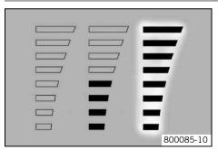
The temperature display consists of 8 bars. The more bars that light up, the hotter the coolant. When the upper bar lights up, all bars in the display begin to flash and the temperature warning lamp lights up.
