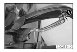
Push the hand brake to the handlebar and check free travel •.
