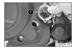
Remove the oil filler plug with O-ring • from the clutch cover and fill up with engine
