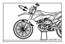
Move the handlebar to the straight-ahead position. Move the fork legs to and fro in the direction of travel.
