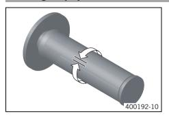
Move the handlebar to the straight-ahead position. Move the throttle grip backwards and forwards to ascertain the play in the throttle cable.
