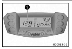
The speed **1** is shown in kilometers per hour **km/h** or in miles per hour **mph**.
