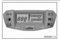
When you switch on the ignition, all display segments light up for a second as a function test.
