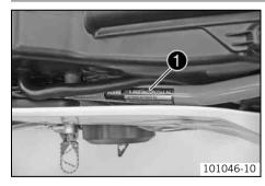
Type label • is located on the upper right frame tube below the seat.
