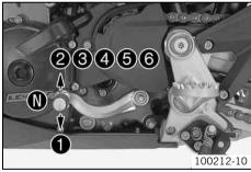
The gear positions can be seen in the photograph. The neutral or idle position is between the first and second gears.
