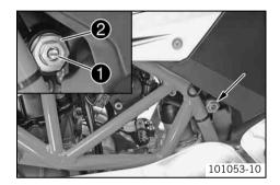
Turn the adjusting screw • clockwise with a screwdriver up to the last perceptible click.
