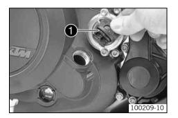
Remove filler plug with O-ring • from the clutch cover and add engine oil.
