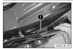
Type label • is located on the upper right frame tube below the seat.
