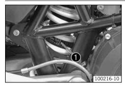
The shock absorber part number  $oldsymbol{0}$  is on the right of the shock absorber.
