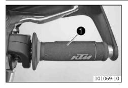
The throttle grip • is fitted on the right side of the handlebar.
