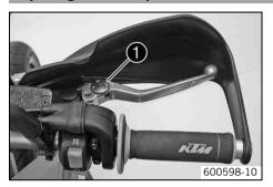
Adjust the basic setting of the hand brake lever to your hand size by turning adjusting wheel •.
