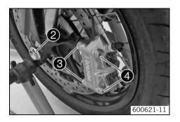
Clean and grease the thread of the wheel spindle and screw ②.
