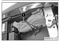
The tool set  $\bullet$  is located in the storage compartment under the seat.
