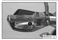
The horn button  $\bullet$  is fitted on the left side of the handlebar.
