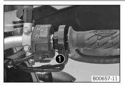
The electric starter button  $\bullet$  is fitted on the right side of the handlebar.
