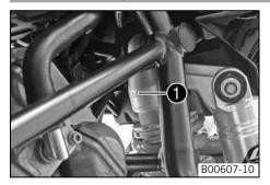
The shock absorber part number  $\bullet$  is stamped on the top of the shock absorber above the adjusting ring on the engine side.
