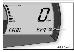
The ice symbol  $\circledast$  lights up to indicate an increased danger of slippery roads. The ice symbol  $\circledast$  appears in the display when the ambient temperature drops below the specified value.
