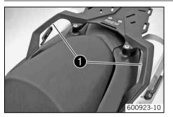
The handrails  $\bullet$  are used for moving the motorcycle around. If you carry a passenger, the passenger can hold onto the handrails during the trip.
