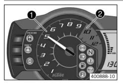
The tachometer **1** shows the engine speed in revolutions per minute. The red marking **2** shows the excess speed range of the engine.
