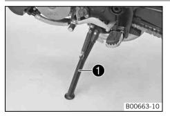
The side stand **①** is located on the left side of the vehicle. The side stand is used to park the motorcycle.
