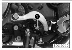
The engine number  $\mathbf{0}$  is stamped on the left side of the engine under the engine sprocket.
