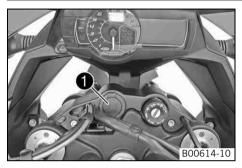
Socket **1** for electrical accessories is fitted next to the ignition/steering wheel lock on the left.
