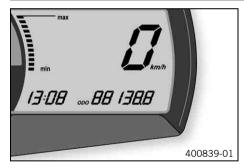
In the **ODO** display mode, the total distance traveled is shown in kilometers or miles.
