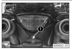
Seat lock ● is located at the rear under the tail light. It can be locked with the ignition key.
