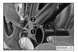
Release nut ① and turn push rod ② until the foot brake lever is in the desired position.
