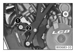
Remove plug **1** and add engine oil to the top marking **2**.
