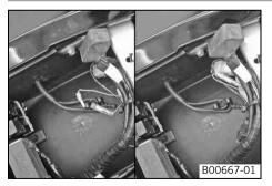
The plug-in connection is located under the seat in front of the tail light. By disconnecting the plug-in connector, the ignition curve for fuel with an octane rating below 95 (ROZ 95/RON 95/PON 91) is activated. While the engine will have a slightly lower power output, this setting prevents engine damage by hindering spark knocking due to poor fuel quality.
