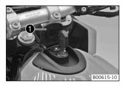
– Lift the cover of the filler cap ① and insert the ignition key.
