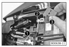
Position the battery in the battery rack. \_
