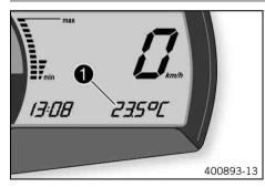
The ambient temperature **①** is displayed in °C or °F.
