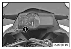
The hazard warning flasher switch  $\bullet$  is fitted next to the combination instrument on the left.
