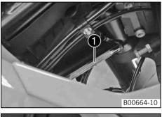
The chassis number **1** is stamped on the frame behind the steering head on the right.
