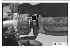
The emergency OFF switch **1** is fitted on the right side of the handlebar.
