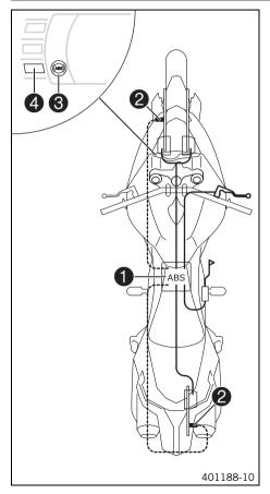
The ABS unit ①, which consists of a hydraulic unit, ABS control unit, and return pump, is installed under the seat. The front and rear wheels each have a wheel speed sensor ②.
