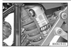
The compression damping of the shock absorber is divided into two ranges: high-speed and low-speed.
