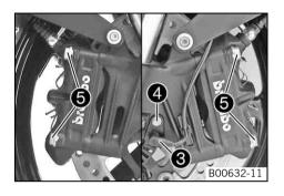
Slide the sleeve onto the wheel speed sensor ③ and push them into the hole together. Mount and tighten screw ④.
