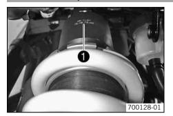
The shock absorber part number  $\bullet$  is stamped on the top of the shock absorber above the adjusting ring toward the rear.
