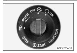
The ignition/steering lock • is in front of the upper triple clamp.
