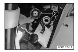
Screw off the radiator cap 2 and check the coolant level in the radiator.
