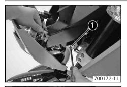
Position the headlight mask. Mount and tighten screws • on both sides.
