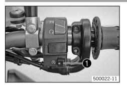
The electric starter button • is fitted on the right side of the handlebar.
