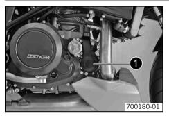
The water pump • in the engine forces the coolant to flow.
