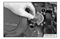
Remove the oil filler plug with O-ring • from the clutch cover and fill up with engine
