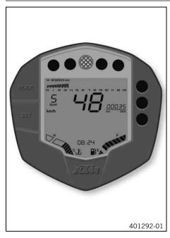
The temperature display consists of 13 bars. The more bars that light up, the hotter the coolant. When all bars light up, the following warning note appears on the info display: **High Coolant Temperature**.
