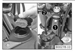
Replace the filler cap and turn clockwise until the release button • locks in place.
