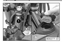
Press release button •, turn filler cap counterclockwise and lift it upwards and remove.
