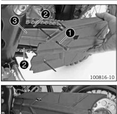
Position the chain guard. Mount cable binder ①.
