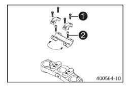
Remove the four screws **1**. Remove the handlebar clamp. Remove the handlebar and lay it to one side.
