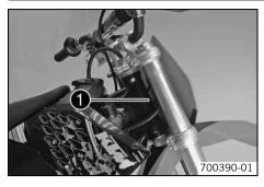
The chassis number **1** is stamped on right of the steering head.
