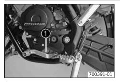
The engine number  ${\ensuremath{\bullet}}$  is stamped on the left side of the engine under the engine sprocket.
