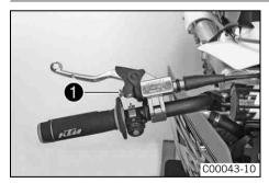
Adjust the basic position of the clutch lever to the size of the rider's hand using adjusting screw ①.
