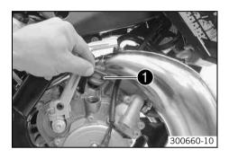
Remove screw cap **1** and fill up with gear oil.
