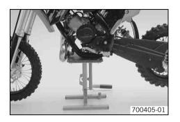
Raise the motorcycle at the frame underneath the engine.
