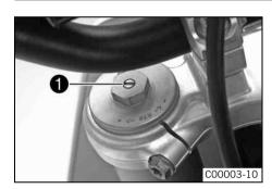
Turn adjusting screw ① clockwise all the way.
