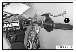
Hand brake lever  $\bullet$  is fitted on the right side of the handlebar. The hand brake lever is used to activate the front brake.
