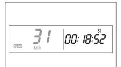
**\$1** (stop watch 1) displays the journey time on the basis of **TR1** and continues when an impulse is received from the wheel speed sensor.
