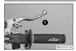
Hand brake lever **1** is located on the right side of the handlebar. The front brake is engaged using the hand brake lever.
