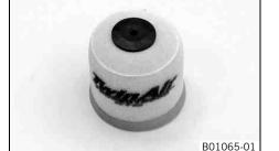
Only press the air filter to dry it, never wring it out.
