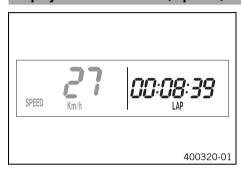
Press the button of briefly and repeatedly until LAP appears at the bottom right of the display.
