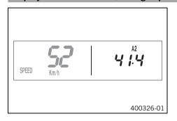
**A2** (average speed 2) shows the average speed on the basis of the current speed if the stop watch **S2** (stop watch 2) is running.
