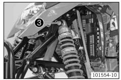
Remove screw 3. Remove the shock absorber.
