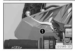
Adjust the basic setting of the clutch lever to your hand size by turning adjusting screw ①.
