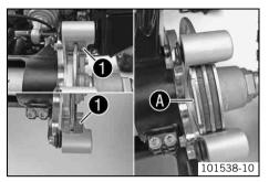
Check that sliding plates • are seated correctly in the brake caliper support and insert the brake linings.
