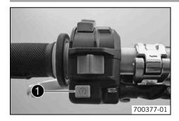
Electric starter button • is fitted on the left side of the handlebar.
