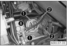
Oil the O-rings of the oil filter covers and mount them with the oil filter covers. Mount and tighten screws • and •.
