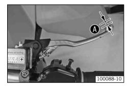
Push the hand brake lever forward and check free travel .
