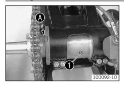
Use a grease gun to fill the rear wheel eccentric element via grease nipple • until grease emerges from the left shaft seal ring •.
