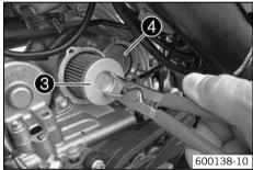
Pull the oil filters 3 and 4 out of the engine case.
