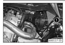
The radiator fan **1** is located on the radiator under the fuel tank.
