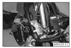
Remove the radiator cap 3. Completely drain the coolant.
