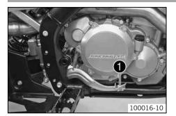
The foot brake lever **1** is located in front of the right footrest and operates the rear wheel brake.
