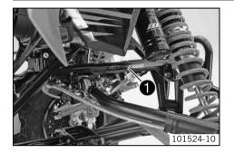
The chassis number lacktriangle is stamped on the right side of the frame in the vicinity of the upper A-arm.
