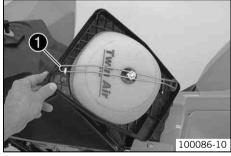
Put in both parts together, position them and fix them with the air filter support 1.
