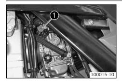
The hot start button (red) • is fitted on the left side of the carburetor.
