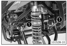
Align the heim joint at right angles to screws ② and tighten nut ①.
