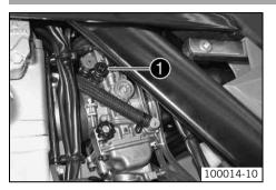
The choke **1** is fitted on the left side of the carburetor.
