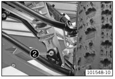
Position the shock absorber in the lower A-arm. Mount and tighten screw ②.
