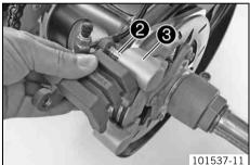
Grease bearing bolt ② and insert the brake caliper with the bearing bolt into the brake caliper support ③.
