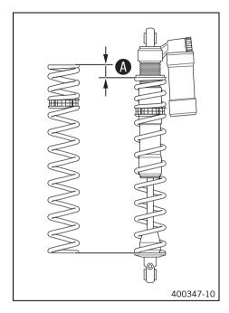
Tighten the spring pack by turning adjusting ring 2 to measurement 4.
