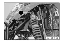
Position the front shock absorber with the reservoir toward the rear. Mount and tighten screw 1.
