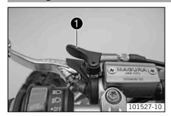
The reverse gear release lever **1** is fitted on the left side of the handlebar.
