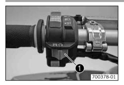
The **ENG. STOP** switch **1** is fitted on the left side of the handlebar.
