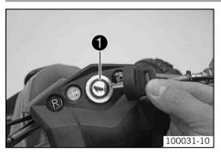
The ignition lock **1** is located on the instrument support.
