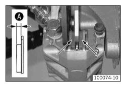
Check the brake linings of both front brake calipers for minimum thickness **3**.
