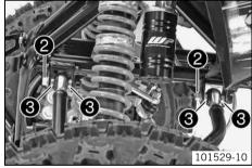
Remove screws 2 with bushings 3.
