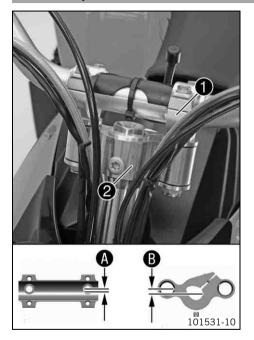
The handlebar position can be adjusted 4-fold by turning the handlebar support **1** and the handlebar support **2**.
