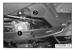
Hook catch • of the radiator spoiler into holder • of the fuel tank and position it on the radiator.
