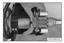
Press the brake caliper onto the brake disc by hand in order to push back the brake piston.
