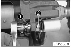
Loosen the screw • while holding the hexagonal head • of the bearing bolt. Unscrew
