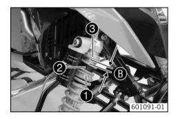
Measure the cross over setting 3 between sliding bushing 2 and the collar of adjusting ring 3.
