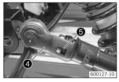
Insert tool 4 in the heim joint and clip onto the A-arm.
