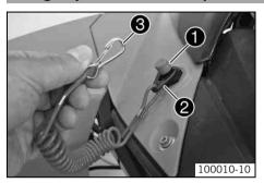
The emergency OFF switch ● is mounted on the left in front of the fuel tank. A rip cord is attached to clip ②. It can be attached to the clothing of the rider by means of carabiner ③. The emergency OFF switch shuts the engine off if the rider falls off the vehicle.
