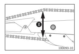
Push the upper chain section at the end of the chain sliding component upwards to measure the chain tension .
