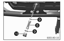
Insert oil screen **3** with O-rings **9** into screw plug **0** and tighten. Guideline
