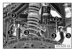
Position the A-arm with bushings **3**. Mount and tighten screws **2**.
