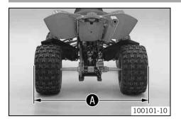
The toe width **4** can be adjusted by installing the spacer in various ways.
