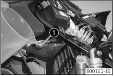
Fill the coolant into the radiator ①.
