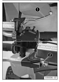
The hand brake lever **1** is located on the right side of the handlebar and operates the front brakes.
