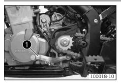
The shift lever • is mounted on the left side of the engine.
