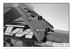
Remove the screws • on the fuel tank.
