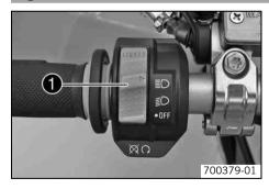
The light switch • is fitted on the left side of the handlebar.
