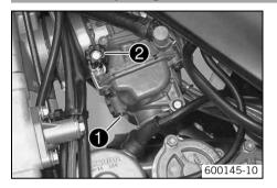
Screw in the idle adjusting screw • until it stops and then to the prescribed basic setting.
