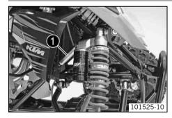
The type label **1** is located on the frame tube on the right in front of the radiator.
