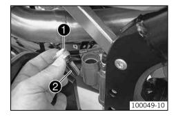
Remove screw cap 1 with membrane 2.
