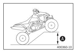
Position the vehicle as shown and secure it against rolling away. The height difference must be achieved.
