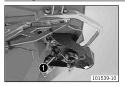
Pull the release hook • back. Lift up the seat at the rear, pull it back and then remove from above.
