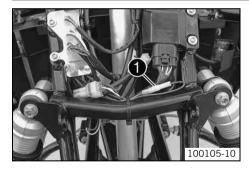
Plug-in connector **1** is located under the trim at the front on the frame tube.
