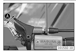
Move the handlebar to the straight-ahead position. Move the reverse gear release lever back and forth slightly to ascertain the play in the cable .
