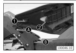
Hook slot ① on the seat into collar sleeve ③ of the fuel tank, lower the rear of the seat and slide tab ② under fuel tank ③.
