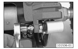
Swing the brake caliper downward. Mount and tighten the screw.
