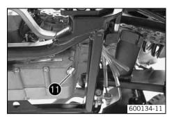
Mount oil drain plug with the seal ring and tighten it.
