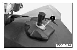
Press release button •, turn filler cap counterclockwise and lift it free.
