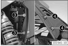
Mount and tighten screws 3 on the radiator.
