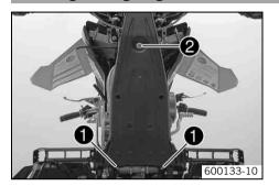
Position the engine guard on the frame bearer. Mount and tighten screws **1** and **2**.
