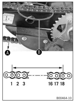
Pull on the lower part of the chain with the specified weight 4.
