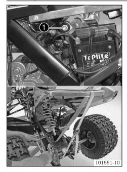
Position the shock absorber in the vehicle with the reservoir on the right. Mount and tighten the top screw ●.
