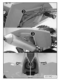
Mount and tighten screws 3.
