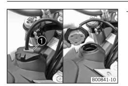
Press release button  $\mathbf{0}$ , turn filler cap counterclockwise and lift it upwards and remove.
