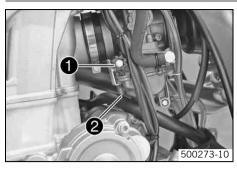
Screw in idle mixture adjusting screw **2** all the way and then turn it to the prescribed basic setting.
