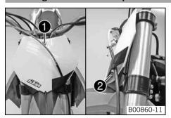
Position the start number plate. Mount and tighten screw ①.
