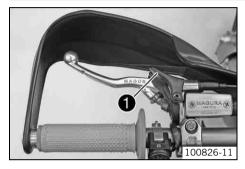
The hot start lever  $\bullet$  is fitted on the left side of the handlebar.
