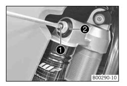
Turn adjusting screw ① clockwise with a screwdriver up to the last perceptible click.
