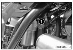
The shock absorber part number  ${\bf 0}$  is stamped on the top of the shock absorber above the adjusting ring on the engine side.
