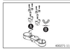
On the upper triple clamp, there are 2 holes at a distance of ( to each other.
