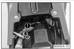
The plug connection  $\bullet$  is located under the seat near the upper shock absorber fixation.
