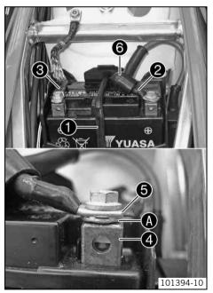
Insert the battery into the battery compartment with the terminals facing to the front.
