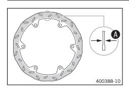
Check the thickness of the front and rear brake discs at several places on the disk to see if it conforms to measurement ④.
