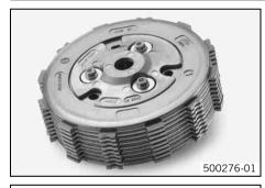
The antihopping system reduces the force required to activate the clutch and improves clutch handling; in addition, it increases riding stability by reducing slippage of the rear wheel by means of engine braking action during downshifting.
