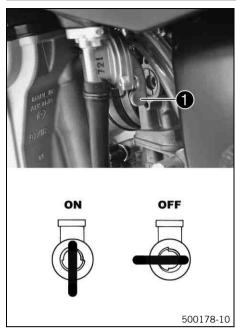
With the tap handle  ${\bf \bullet}$  on the fuel tap, you can open or close the supply of fuel to the carburetor.
