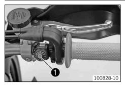
Electric starter button  ${\color{black} \bullet}$  is fitted on the right side of the handlebar.
