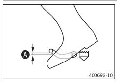
Sit on the vehicle in the riding position and determine the distance <sup>(1)</sup> between the upper edge of your boot and the shift lever.
