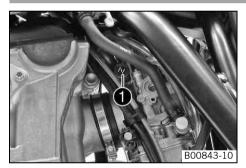
Choke **1** is fitted on the left side of the carburetor. Activating the choke function frees an opening through which the engine can draw extra fuel. This gives a richer fuel-air mixture, which is needed for a cold start.
