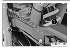
The shock absorber part number lacktriangle is shown on a sticker applied to the shock absorber case.
