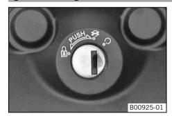
The ignition/steering lock • is located in front of the upper triple clamp.
