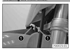
Position the fender with holding lugs • into the drill holes on the start number plate. WORK
