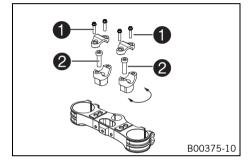
Remove the four screws ①. Remove the handlebar clamps. Remove the handlebar and lay it to one side.
