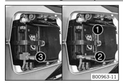
Position the battery in the battery holder.
