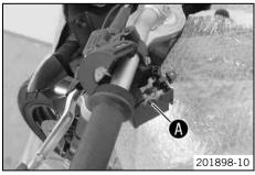
Mount and tighten the rear mirror adapter and rear mirror on both sides.
