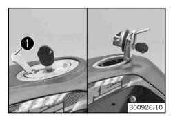
Lift cover • of the filler cap and insert the ignition key in the lock.
