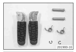
Mount the footrests with the springs and bolts. Secure the pins with the lock rings.
