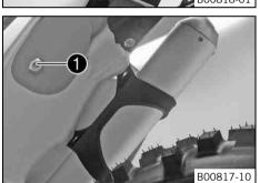
11.24 Removing the air filter box lid
