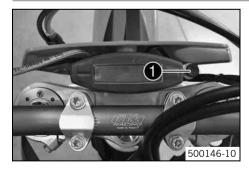
Light switch  $\ensuremath{f 0}$  is located to the right of the speedometer.
