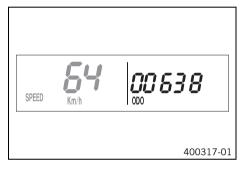
Press the button O briefly and repeatedly until ODO appears at the bottom right of the display.
