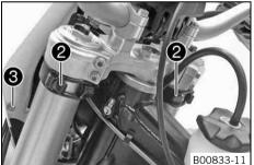
Position the headlight mask and fix it with the rubber band **2**.
