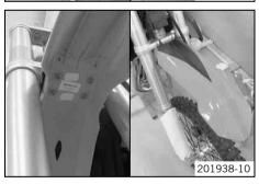
Position the fender. Mount and tighten screws.
