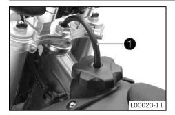
Mount filler cap and turn it clockwise until the fuel tank is tightly closed.
