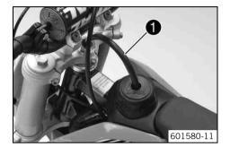
Put the tank cap on and turn it clockwise.
