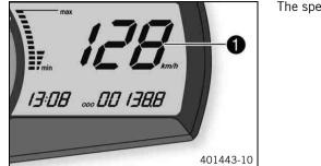
The speed **1** is shown in kilometers per hour **km/h** or in miles per hour **mph**.
