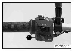
The horn button  $\bullet$  is fitted on the left side of the handlebar.
