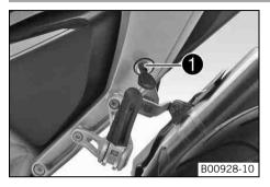
The seat lock  $\bullet$  is located on the left side of the vehicle. It can be locked with the ignition key.
