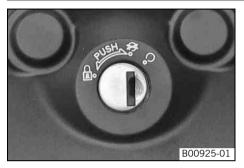
The ignition/steering lock **1** is located in front of the upper triple clamp.
