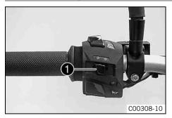
The turn signal switch **1** is fitted on the left side of the handlebar.
