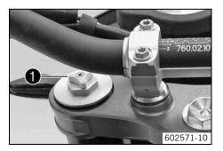
– Turn the white adjusting screw **1** all the way clockwise.
