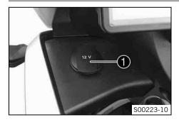
Socket **①** for electrical accessories is fitted to the left of the combination instrument. It is connected to permanent positive and fuse-protected.
