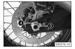
Remove nut **3**. Remove chain adjuster **4**.
