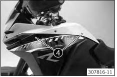
Mount and tighten screws **4**.
