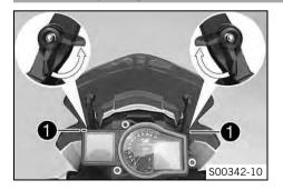
Release clamping lever • by pulling in the direction of the arrow.
