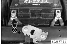
Disconnect the negative cable of the battery to avoid damage to the motorcycle's electronics.
