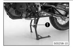
In addition to the side stand, the vehicle is equipped with a center stand **①**.
