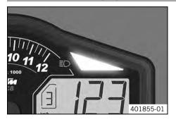
The shift warning light flashes or lights up when the transmission should be shifted. In the **"Shift Light"** menu, the engine speed for the shift warning light can be set. The shift warning light flashes at **"RMP1"** and lights up at **"RPM2"**.
