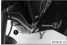
Attach catch • and bracket • of the side cover to the fuel tank and position the side cover.
