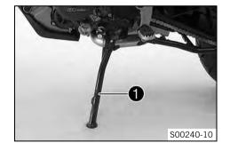
The side stand **①** is located on the left side of the vehicle. The side stand is used for parking the motorcycle.
