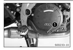
Foot brake lever • is located in front of the right footrest.
