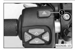
The hazard warning flasher switch • is fitted on the combination switch on the left. The hazard warning flasher is used to indicate emergency situations.
