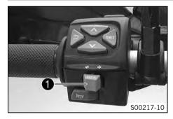
The turn signal switch **1** is fitted on the combination switch on the left.
