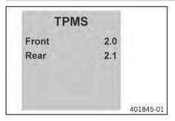
Press the UP or DOWN button until the "TPMS" menu appears on the matrix display.
