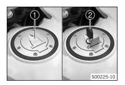
Lift cover • of the filler cap and insert ignition key • in the fuel tank lock.
