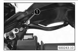
Adjust the basic position of the hand brake lever to your hand size by turning adjusting wheel •.
