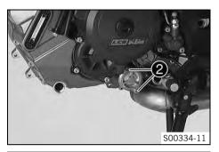
Mount and tighten screws ②.
