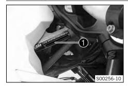
The type label • is on the top right of the frame behind the steering head.
