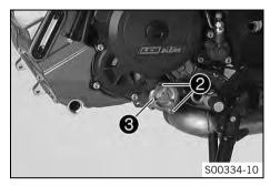
Remove screws 2. Remove the oil filter cover 3 with the O-ring.
