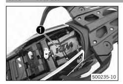
The tool set **1** is located in the storage compartment under the seat.
