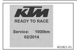
The matrix display is controlled using the menu switch ( p. 26). After the ignition is switched on, the display shows when the next service ( p. 44) is due. If the General warning lamp I lights up among the indicator lamps ( p. 41), the corresponding message appears in the matrix display. The **Set** button is used to confirm receipt of the information and the message is cleared.
