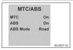
The traction control lowers the tightening torque in case of loss of traction in the rear wheel. Depending on the traction control setting, a slight slip on the rear wheel may be desirable. Example: Offroad.
