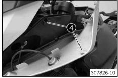
Pull the mask spoiler upward from bracket 4.
