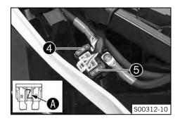
Remove the faulty main fuse 4.
