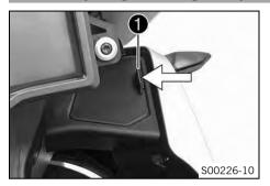
Press button ● in the direction of the arrow and lift the cover at the same time.
