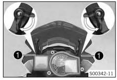
Lock clamping lever • by pushing in the direction of the arrow.
