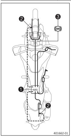
The ABS unit ①, which consists of a hydraulic unit, ABS control unit, and return pump, is installed under the seat. A wheel speed sensor ② is located at the front and rear wheels.
