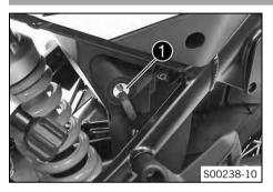
The seat lock **1** is located on the left side of the vehicle. It can be unlocked using the ignition key.
