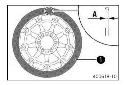
Check the thickness of the front and rear brake discs at multiple points on each brake disc to ensure it is at least thickness .
