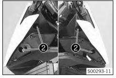
Mount and tighten screws 2.
