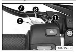
The light switch • is fitted on the combination switch on the left.
