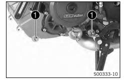
Mount and tighten oil drain plugs • with the magnet, O-rings, and oil screen.
