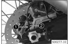
Remove screw • and pull wheel speed sensor • out of the hole.
