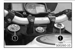
Turn adjusting screws ● counterclockwise all the way.
