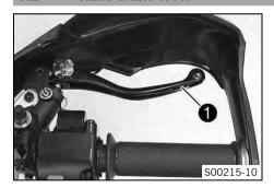
The hand brake lever • is fitted on the right side of the handlebar.
