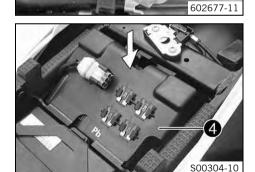
Fold down cover 4 and let it lock by pushing down lightly.
