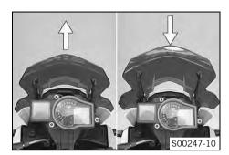
Move the wind shield in the required position.
