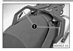
The handrails **①** are used for moving the motorcycle around. If you carry a passenger, the passenger can hold onto the handrails during the trip.
