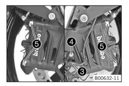
Slide the sleeve onto the wheel speed sensor 3 and push them into the hole together.
