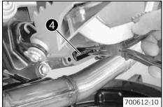
Pull oil screen 4 out of the engine case with pliers.
