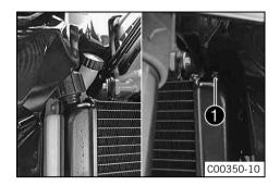
Remove the radiator cap and pour in coolant until it emerges without bubbles at the vent hole, and then immediately mount and tighten the bleeder screw 1.
