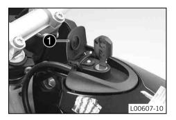
Lift the cover of the filler cap • and insert the ignition key.
