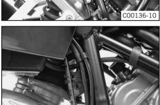
Remove screw • and take off the brake line guide.
