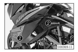
Position the spoilers on both sides. Mount and tighten screws 2.
