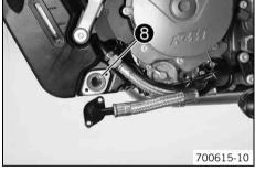
Pull oil screen 8 out of the oil tank.
