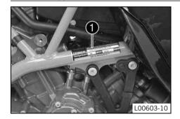
Type label **1** is located on the upper frame tube on the right.
