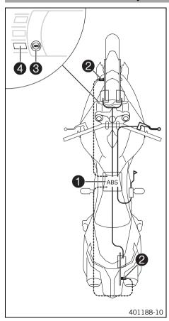
The ABS unit ①, which consists of a hydraulic unit, ABS control unit, and return pump, is installed under the seat. The front and rear wheels each have a wheel speed sensor ②.
