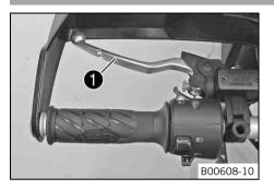
The clutch lever • is fitted on the left side of the handlebar. The clutch is hydraulically operated and self-adjusting.
