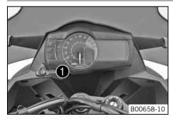
The hazard warning flasher switch • is fitted next to the combination instrument on the left.
