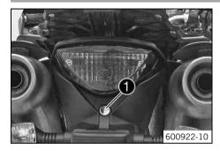
Seat lock • is located at the rear under the tail light. It can be locked with the ignition key.
