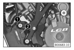
Remove plug • and add engine oil to the top marking •.
