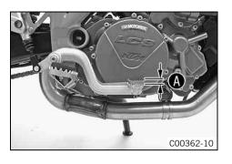
Move the foot brake lever back and forth between the end stop and the contact to the piston rod and check free travel **(4)**.
