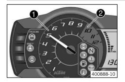
The tachometer • shows the engine speed in revolutions per minute.
