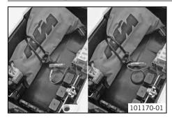
The plug-in connection is located under the seat in front of the tail light. By disconnecting the plug-in connector, the ignition curve for fuel with an octane rating
