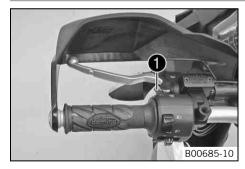
The headlight flasher switch **1** is fitted on the left side of the handlebar.
