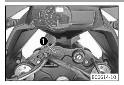
Socket • for electrical accessories is fitted next to the ignition/steering wheel lock on the left.
