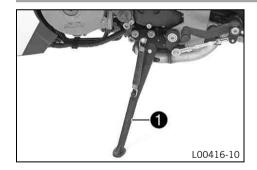
The side stand **①** is located on the left side of the vehicle. The side stand is used to park the motorcycle.
