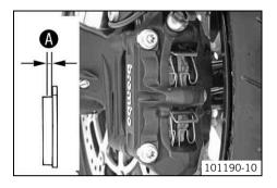
Check all brake linings on both brake calipers to ensure they have minimum thickness .
