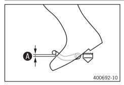
Sit on the vehicle in the riding position and determine the distance between the upper edge of your boot and the shift lever.
