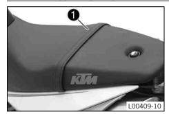
Supporting strap • is mounted on the seat.
