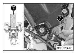
Pull oil sieve out of the oil tank.
