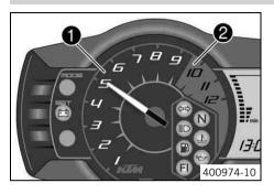
The tachometer **1** shows the engine speed in revolutions per minute.
