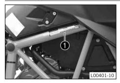
Type label **1** is located on the upper frame tube on the right.
