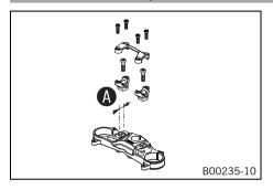
On the upper triple clamp are two holes a distance of **4** apart.
