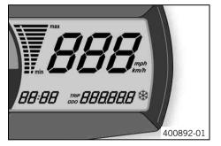
When you switch on the ignition, all display segments light up for one second as a function check.
