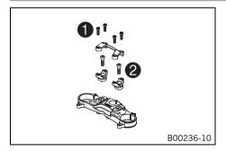
Remove the four screws ①. Remove the handlebar clamp. Take off the handlebar and set it aside.
