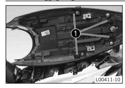
Baggage lugs • are located on the underside of the seat.
