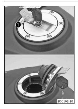
Lift the cover ● of the filler cap and insert the ignition key in the lock.
