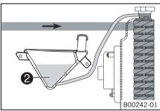
Cooling takes place by means of the air stream and a radiator fan, which is controlled by a thermoswitch.
