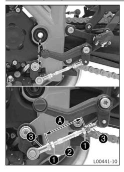
Release nuts • and turn shift rod • until the shift lever is in the desired position.
