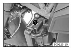
Remove the radiator cap and pour in coolant until it emerges without bubbles at the vent hole, and then immediately mount and tighten the bleeder screw ①.
