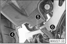
Position oil line **6**. Mount and tighten screws **6**.
