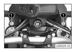
Position the headlight mask. Mount and tighten screws ①.
