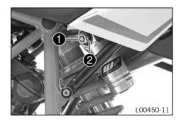
Turn adjusting screw ① clockwise all the way using a socket wrench.
