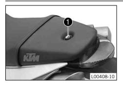
Seat lock **①** is located at the rear of the seat. It can be locked with the ignition key.
