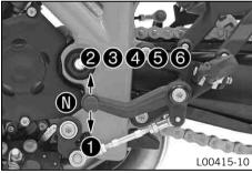
The gear positions can be seen in the photograph. The neutral or idle position  $\mathbf{0}$  is between the first and second gear.
