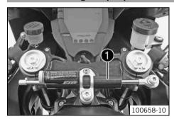
The steering damper part number • is stamped on the top of the steering damper.
