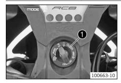
The ignition/steering lock • is located in front of the upper triple clamp.
