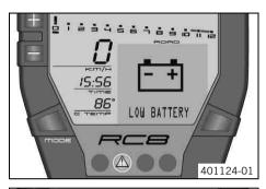
**LOW BATTERY** appears on the info display if the battery voltage falls below the specified value.
