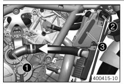
The water pump with a 3D water pump wheel • in the engine ensures forced circulation of the coolant. The heat exchanger enables faster warming of the engine oil at the start of a journey and better heat dissipation for the engine oil during the journey.
