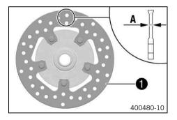
Check the thickness of the brake disc in several places to see if it conforms to measurement .
