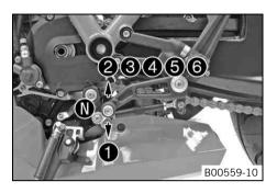
The gear positions can be seen in the picture. The neutral or idle position  $\mathbf{0}$  is between the first and second gear.
