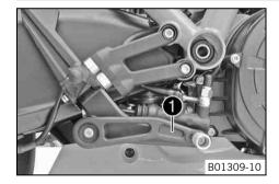
The foot brake lever **①** is in front of the right footrest. The foot brake lever operates the rear brake.
