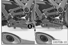
Check the foot brake lever setting.
