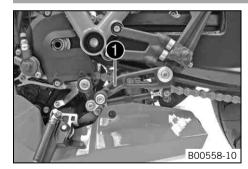
The shift lever • is mounted on the left of the engine.
