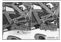
The adjustable footrest system enables an individual setting of the footrest height and an individual adjustment of the controls.
