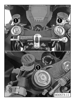
Turn adjusting screws • clockwise to the stop.
