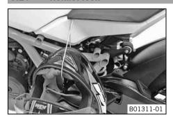
The steel cable in the tool set can be used to lock a helmet to the vehicle to prevent it from being stolen.
