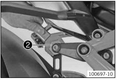
Turn eccentric shaft ② to the desired position using the tool from the tool set.
