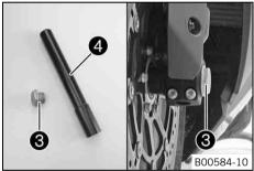
Insert the wide spacer on the left-hand side ② (when looking in the direction of travel).
