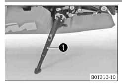
The side stand **1** is located on the left side of the vehicle. The side stand is used for parking the motorcycle.
