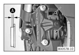
Check all brake linings on both brake calipers to ensure they have minimum thickness .
