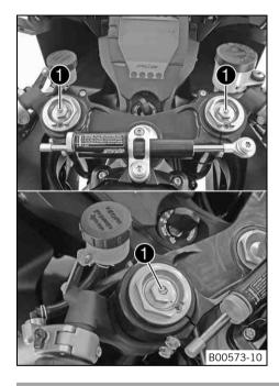
Turn adjusting screws • clockwise to the stop.
