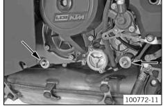
Mount and tighten the oil drain plugs with the magnet, O-rings, and oil screen. Guideline
