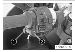
The **MODE** button **1** is fitted on the handlebar, front left.
