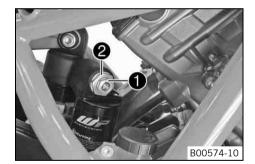
Turn adjusting screw 1 clockwise all the way using a socket wrench.
