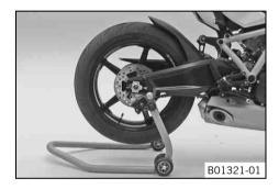
Insert the adapter into the lifting gear at the rear.
