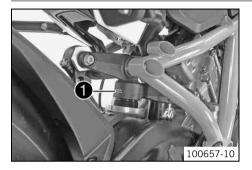
The shock absorber part number  $\bullet$  is stamped on the upper part of the shock absorber above the adjusting ring towards the rear.
