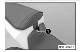
The seat lock **1** is behind the seat. It can be locked with the ignition key.
