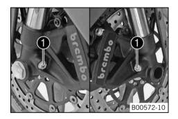
Turn adjusting screws • clockwise to the stop.
