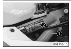
The vehicle identification number lacktriangle is stamped on the frame behind the steering head on the right.
