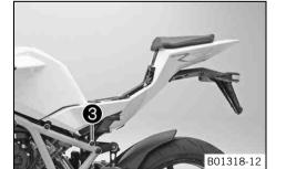
Tighten screws 3 on the left and right sides of the vehicle.
