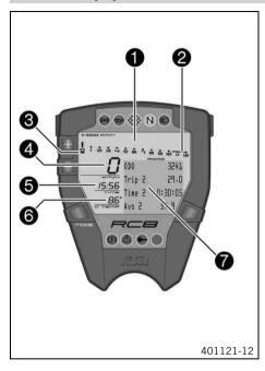
The tachometer **1** displays the engine speed in revolutions per minute (RPM). The red marking **2** marks the over-rev (excessive speed) range of the engine. The gear display **3** shows the engaged gear.
