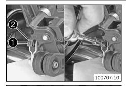
Use the tool to press in the anti-rotation lock ②, then turn the piston rod ①.
