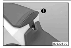
The supporting strap **1** is provided for the passenger to hold on to.
