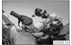
Remove the controls from the transport holder. Remove the screws and handlebar clamps. Remove the transport holder.
