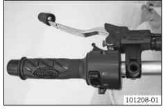
Position the clutch master cylinder and tighten the screw.
