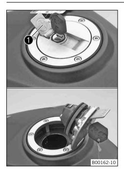
Lift the cover **1** of the filler cap and insert the ignition key in the lock.
