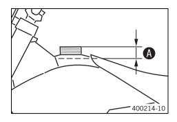
Fill the fuel tank with fuel up to measurement ①.
