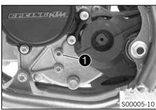
Remove gear oil level check screw ①.
