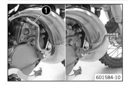
The kickstarter **1** is fitted on the right of the engine.
