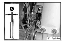
Check the brake linings for minimum thickness •.
