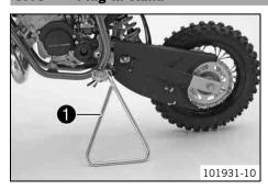
The fixture for the plug-in stand lacktriangle is located on the frame on the left side of the vehicle.
