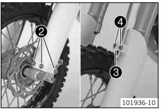
Position the fork protection on the left fork leg. Mount and tighten screws 2.
