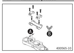
On the upper triple clamp, there are 2 holes at a distance of **1** to each other.
