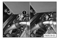
The choke lever **1** is fitted on the right of the carburetor.
