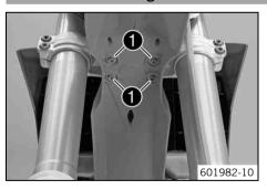
Remove screws ①. Remove the front fender.
