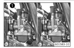
The choke knob • is fitted on the left of the carburetor.
