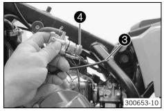
Turn the oil pump gear 4 counterclockwise until oil flows out of oil line 8 without bubbles.
