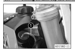
Put the oil tank cap on and turn it clockwise.
