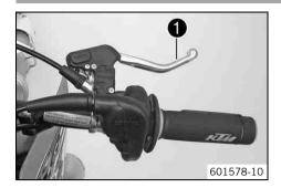
Hand brake lever **1** is fitted on the right side of the handlebar. The hand brake lever is used to activate the front brake.
