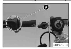
Position the throttle grip so that surface (a) is vertical.
