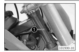
The chassis number **1** is stamped on right of the steering head.
