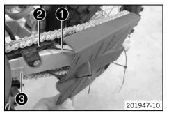
Position the chain guard. Mount cable binder ①.
