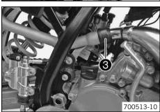
Pull the main silencer off of the manifold at the rubber sleeve 3.
