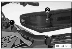
Hook the seat onto screw • and lower the seat at the rear while pushing it forward.
