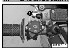
The kill switch **1** is fitted on the left side of the handlebar.
