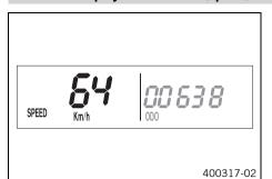
The current speed is displayed in the **SPEED** display mode.
