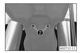
Mount and tighten screws ②.
