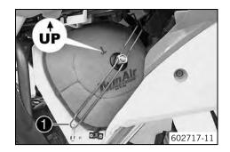
Insert both parts together, position them and fasten them using air filter holder **①**.
