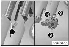
Position the brake caliper. Mount and tighten screws 9.
