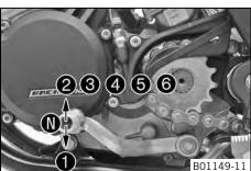
The gear positions can be seen in the photograph.
