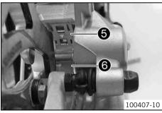
Check that leaf spring 6 in the brake caliper and sliding plate 6 in the brake caliper support are seated correctly.
