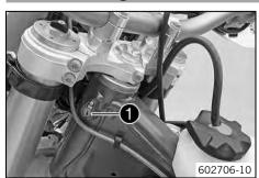
Steering lock lacktriangle is fitted on the left side of the steering head. The steering lock is used to lock the steering. Steering, and therefore riding, is no longer possible.
