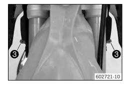
Pull both spoilers off of the sides of the radiator bracket 3 and lift off the fuel tank.
