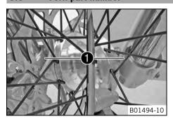
The fork part number • is stamped on the inner side of the fork stub.
