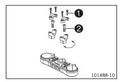
Remove screws ①. Remove the handlebar clamp. Remove the handlebar and lay it to one side.
