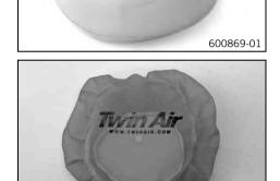
Mount the dust cover for the air filter for sand.
