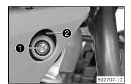
Turn adjusting screw • clockwise with a screwdriver to the last click.
