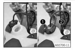
Replace the filler cap and turn clockwise until the release button 1 locks in place.
