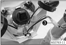
Disconnect the electrical plug-in connection 3 and take off the headlight mask with the headlight.
