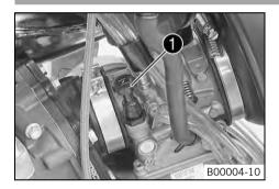
The choke lever **1** is fitted on the left side of the carburetor.
