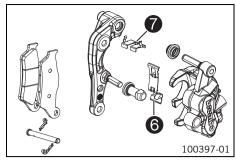
Check that leaf spring • in the brake caliper and sliding plate • in the brake caliper support are seated correctly.
