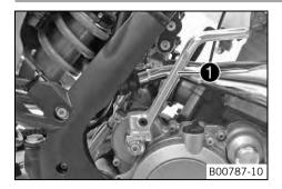
The kick starter  $oldsymbol{0}$  is fitted on the right side of the engine. The top part can be swiveled.
