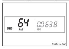
Press the button of briefly and repeatedly until SPEED appears on the left side of the display.
