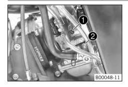
Screw in idle air adjusting screw 2 all the way and turn it to the specified basic position.
