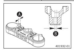
On the upper triple clamp, there are two holes a distance of **4** apart.
