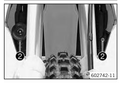
Mount and tighten screws ② with the collar sleeve.
