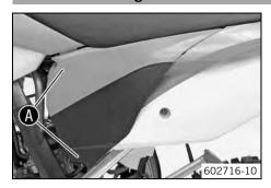
Pull off the air filter box lid in area sideways and remove it toward the front.
