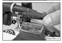
Correct the brake fluid quantity to level **3**.
