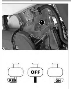
The fuel tap is on the left side of the fuel tank.
