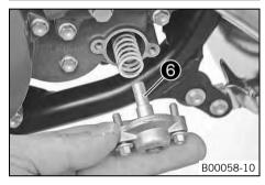
Mount the required auxiliary spring 4 and adjusting spring 5 and slide them into the clutch cover together.
