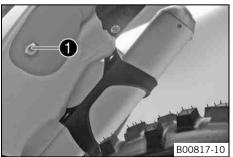
Mount and tighten screw • of the seat fixation.
