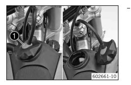
Press release button **1**, turn the filler cap counterclockwise, and lift it free.
