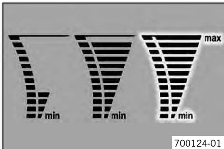
The temperature display consists of 12 bars. The more bars that light up, the hotter the coolant. When the upper bar lights up, all bars in the display begin to flash and the temperature warning lamp lights up.
