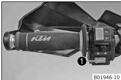
The horn button ❶ is fitted on the left side of the handlebar.
