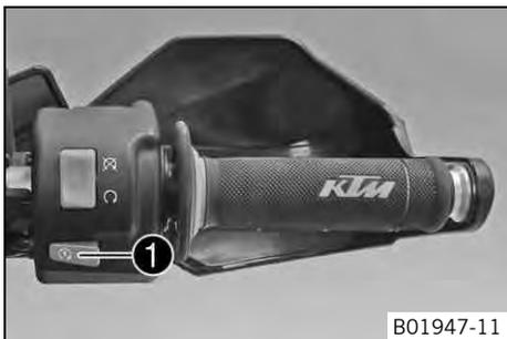
The electric starter button ① is fitted on the right side of the handlebar.
