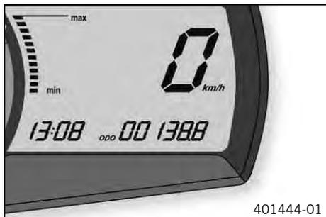
In the **ODO** display mode, the total distance traveled is shown in kilometers or miles.
