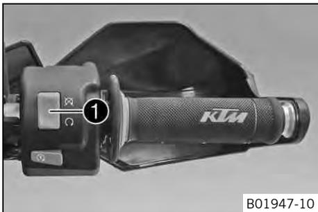
The emergency OFF switch ① is fitted on the right side of the handlebar.
