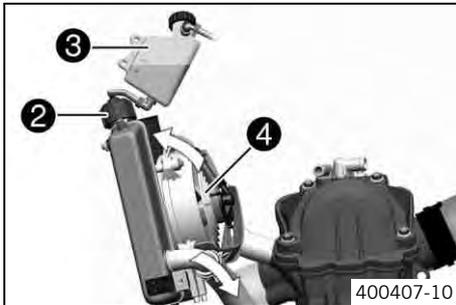
Cooling takes place by means of the air stream and a radiator fan ④, which is controlled by a thermostitch.
