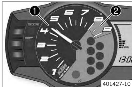
The tachometer **1** shows the engine speed in revolutions per minute.
