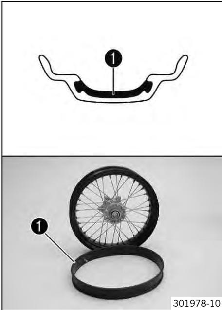
This vehicle makes use of a tubeless tire system in which a tubeless sealing profile **1** is used instead of the conventional tube.
