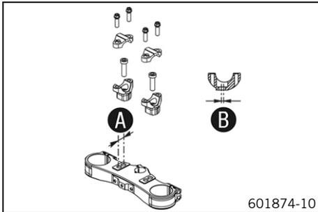
In the upper triple clamp, there are 2 drill holes separated by a distance of **A**.
