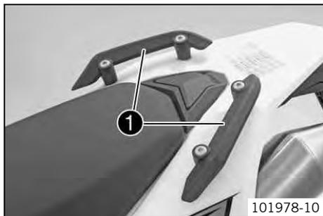
The handrails **1** are used for moving the motorcycle around.
