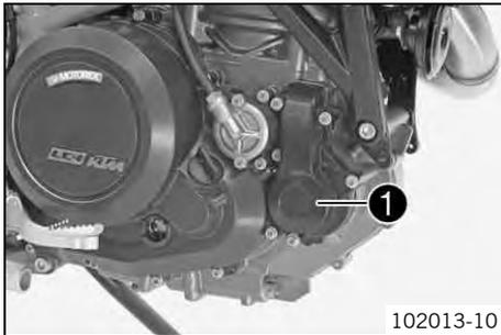
The water pump ① in the engine forces the coolant to flow.
