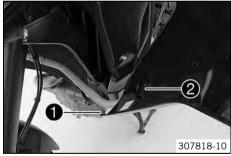
Attach catch 1 and bracket 2 of the side cover to the fuel tank and position the side cover.
