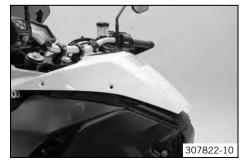
Raise the tank cover at the rear and remove it in a forward direction.
