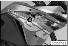
Mount and tighten screws 4.
