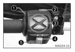
The combination switch is fitted on the left side of the handlebar.
