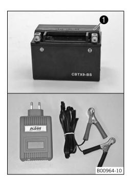
Disconnect the negative cable of the battery to avoid damage to the motorcycle's electronics.
